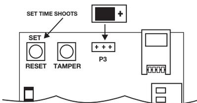
To set the shooting time, after opening the cylinders compartment door, at the top of the PCB, facing the board you must move the jumper P3 in “setting” position.
