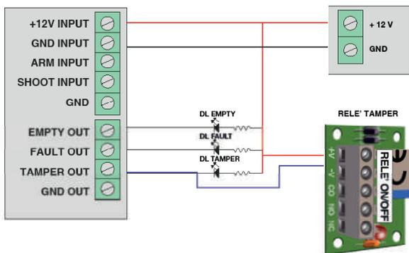
In case of an empty cylinder, the DL EMPTY led will switch on.
