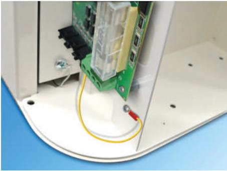
While connecting the machine to the mains power, it is recommended to never disconnect existing ground cable. The fact of disconnecting or modifying existing cables voids the warranty and can cause troubles or accidents related to the temperature control. Connect ground cable from the system to the screw on the metal sheet.
